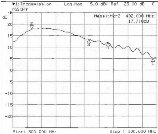
Fig 23: Network analyser plot of the IF amplifier after modification.
