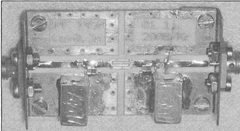
Fig 15: The simulations converted into a prototype with SMA connectors. The circuit must now be measured on the network analyser.
