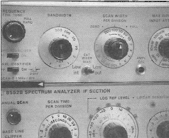
Fig 5: Arrangement of the new switch on the front panel.
